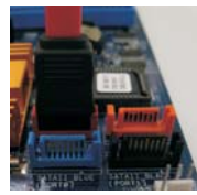
Connect the SATA data cable to the red SATAII connector (SATAII_RED (PORT2))
